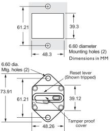
Gasket Part Number: B156-7003-J Material: Black Santoprene. Notes: Optional flange mount gasket for through wall applications. Gasket wraps around breaker to provide a seal between the circuit breaker housing and the panel.
